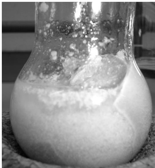
Figure 3. Impression of the gel-like reaction mixtures obtained after suspension polymerization in a high ionic liquid content aqueous phase (Expts 3, 5, and 7).
